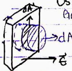
$$\begin{aligned} \Phi_{\text{Tot}} &= \Phi_{A\text{Tot}} + \Phi_{A'\text{Tot}} \\ &= \int_{A\text{Tot}} \vec{E} \cdot d\vec{A} = \vec{E} \int_{A\text{Tot}} d\vec{A} = 2\vec{E} \int_A d\vec{A} = 2EA \end{aligned}$$
